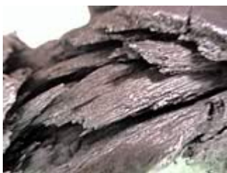
Extrusion: Close-up view of the deformed aluminum
