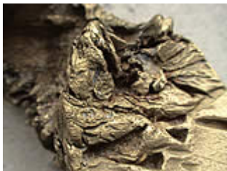
Brass: Close-up view of massive surface erosion.
